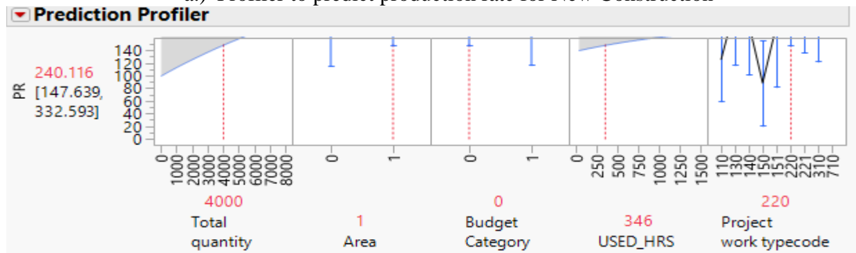
b.) Profiler to predict production rate for Bridge Replacement
